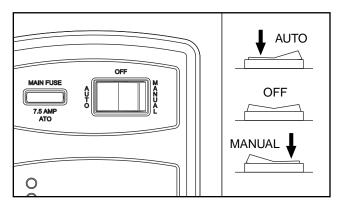
Figure 1. AUTO-OFF-MANUAL Switch Positions
